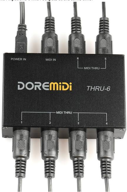
Note: According to the situation, you can choose whether to supply power to the product through POWER IN. In most cases, if you connect 3 or 4 MIDI THRUs, you don't need to supply power. However, whether power is supplied or not depends on whether the power of MIDI IN is sufficient.
